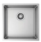
Material AISI 316 L Finishing Brushed R 10 mm welded Inner corners Overall dimensions 440 × 440 mm 400 × 400 mm Basin dimensions Bowl depth 200 mm Standard Strainer 3 ½" Cabinet size 600 mm Top mount Cod. BI 4040 MR Flush mount Cod. **BG 4040 MR**
